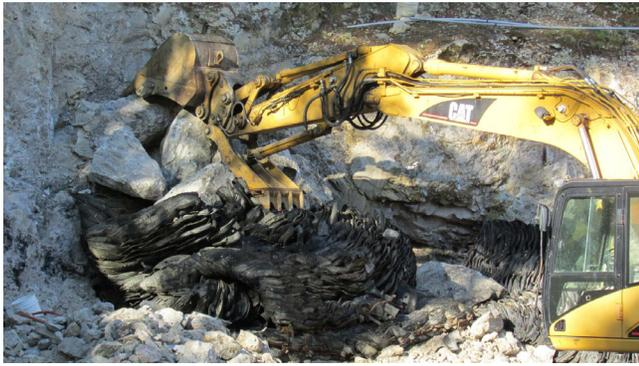
*The excavator at the Havey mine with blast blankets to catch falling debris. Dan Cathey photo.*
