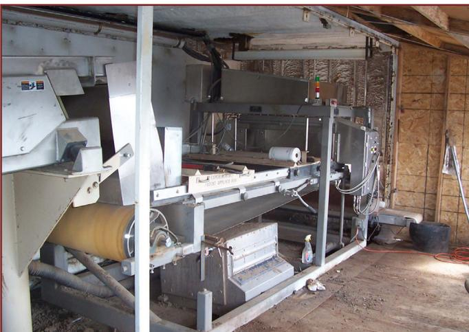
*This optical sorter was being used to increase production at one mine. It replaced a conveyor belt sorting system fondly named "the puker" because human sorters on the belt routinely became sick while watching rocks and sunstones fly by. Jim Landon photo.*
