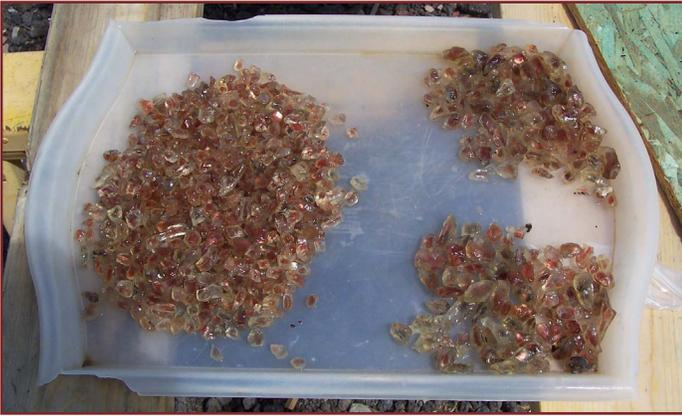
*Mine run rough sunstones are sorted by size and degree of internal color. Clear and lighter colored stones have already been removed. Jim Landon photo.*
